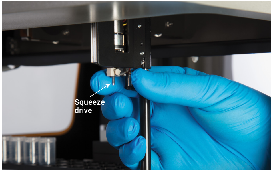
Figure 39. Squeeze Drive. Turn the squeeze drive to release any tools or pipette tips from the pipetting channels.
