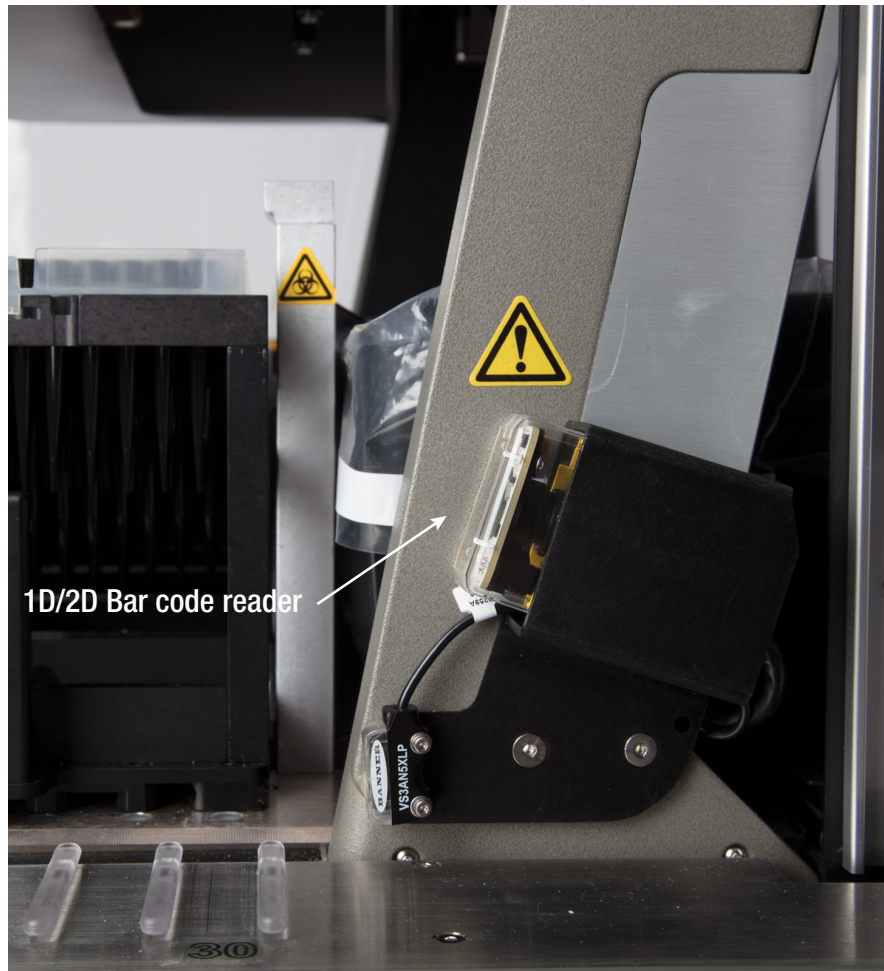
Figure 2. Gantry system on the Maxprep™ Liquid Handler. The gantry system on the Maxprep™ Liquid Handler houses the four pipetting channels on the system. On the front arm of the gantry is the 1D/2D bar code reader.
