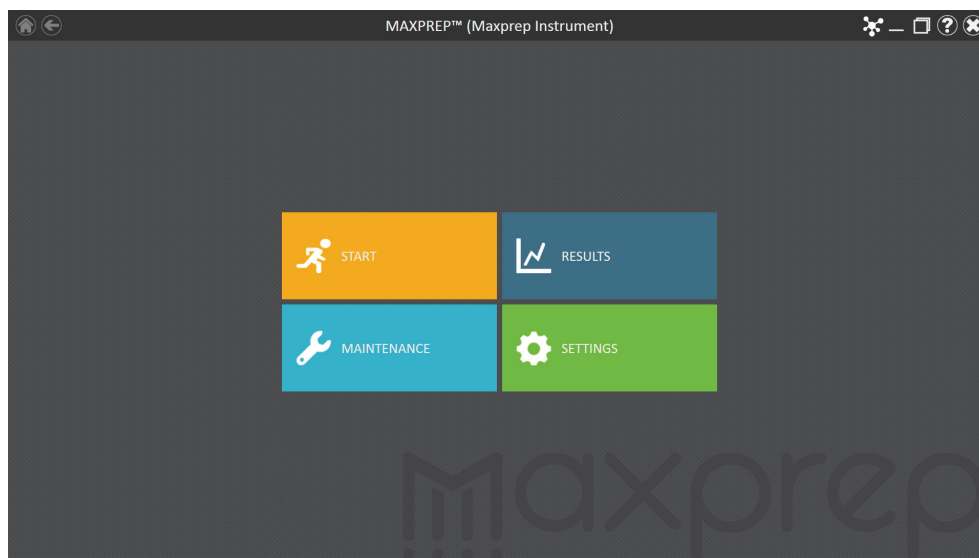
Figure 32. Maxprep™ software 'Home' screen. Selecting the Start button begins the process of running a method on the Maxprep™ Liquid Handler.
